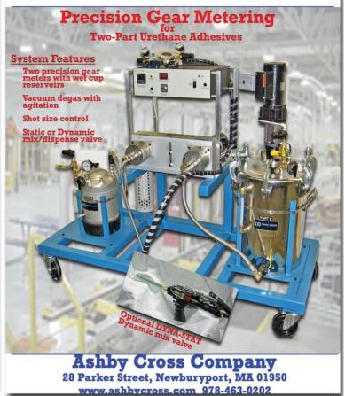
GP80 on a portable cart with 10-gallon and 3-gallon tanks, agitation, and the DYNA-STAT dispense gun
